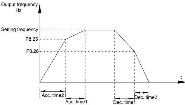
Fig.5-19 Acc./dec. Time switching schematic diagram
