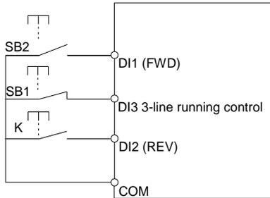
Fig. 5-9 Three-line control mode 2
