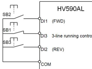
Fig. 5-8 Three-line control mode 1
