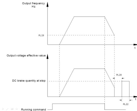
DC brake schematicdiagram
