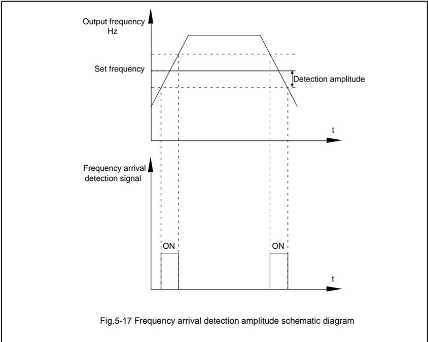
Fig.5-17 Frequency arrival detection amplitude schematic diagram
