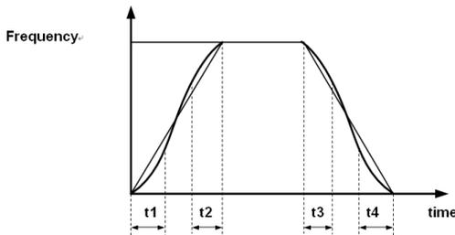
The Figure of S curve acc. /dec. mode C.
