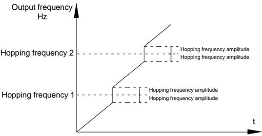
Fig.5-18 Acc./dec. hopping frequency validity schematic diagram
