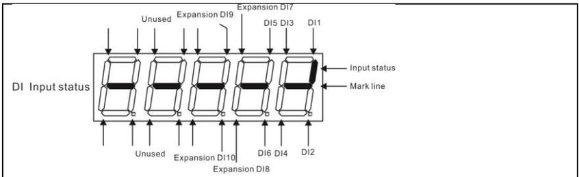
Display DI input status intuitively, offer DI input information more detailed than U0.07, advanced display function.
