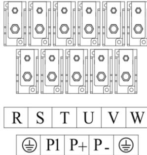
**2.5.2 Main circuit wiring method of the inverter**
