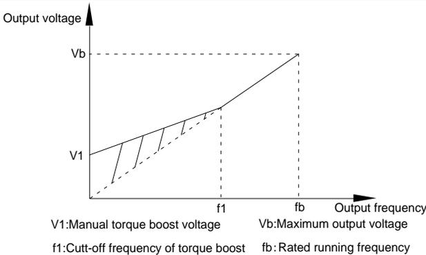
Fig. 5-3 Manual torque boost schematic diagram
