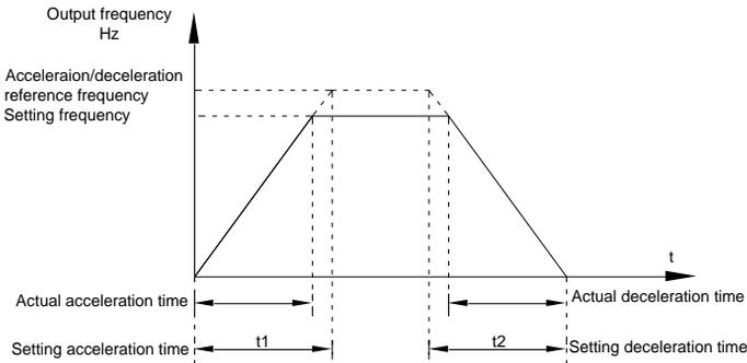
Acceleration/deceleration time schematic diagram
